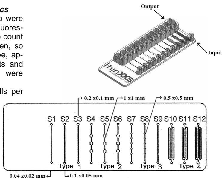
**Fig. 1.** 3D diagram of Thrombi-Chip showing the actual design used in the present study. The lower part of this figure shows Thrombi-Chip channel designs, with dimensions and shapes.
